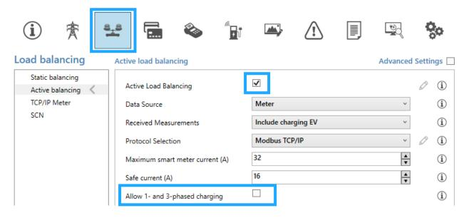
**Note:** the checkbox for 'Allow 1- and 3-phased charging'. This option must be active to allow an Energy Management System to control switching between single-phase and three-phases while charging. In the current implementation this option <u>must</u> be checked locally using the Service Installer Application.
